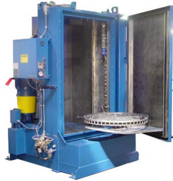
Figure 53 Water blasting cleaning.
