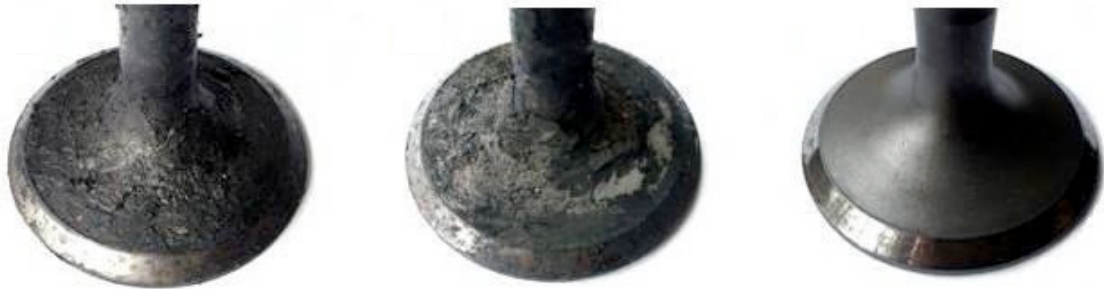
Figure 8 Cleaning an engine valve: part to be remanufactured (a), supercritical cleaning (b), supercritical + water blasting cleaning (c).
