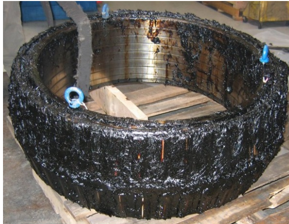
Figure 51 Dirty bearing with grease.
