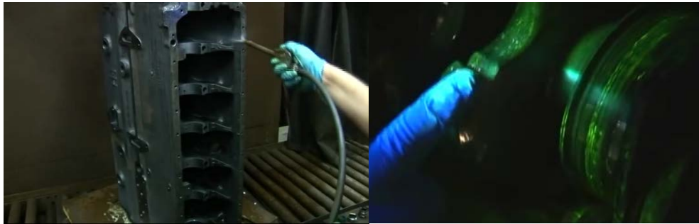
Figure 61 Magnetic particle inspection: engine block (a), crankshaft (b).
