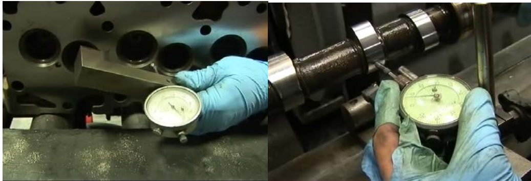
Figure 65 Quality inspection: engine block (a), camshaft (b).
