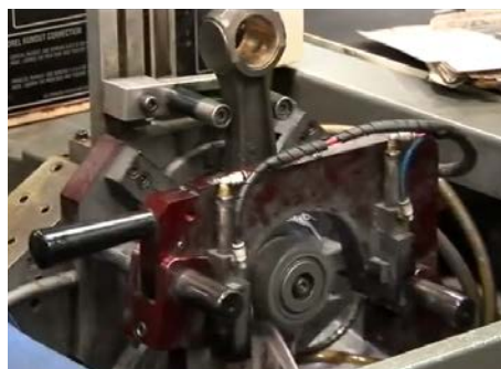
Figure 64 Rod boring operation.
