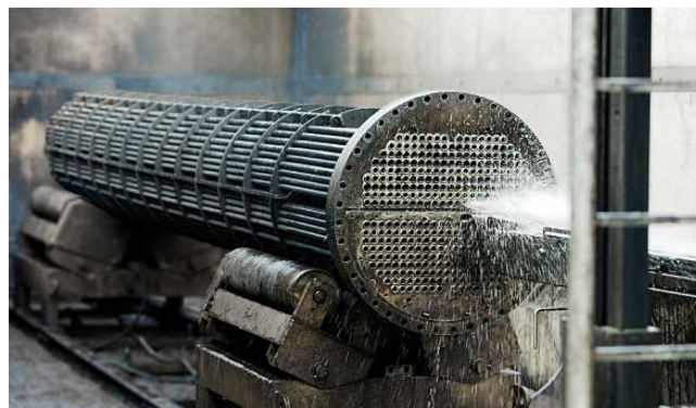
Figure 15 Cleaning a heat exchanger.
