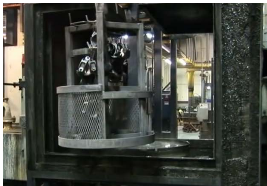
Figure 60 Water blasting cleaning.
