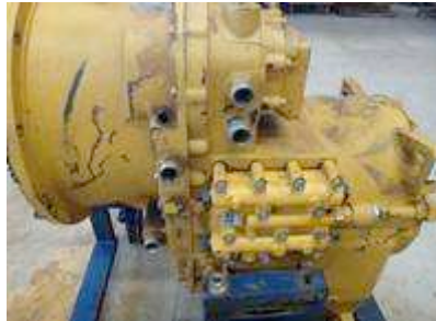
Figure 16 Pre-cleaning of a gear box (water blast cleaning).
