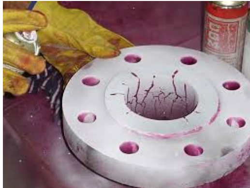
Figure 23 Example of defects (dyes penetrant).
